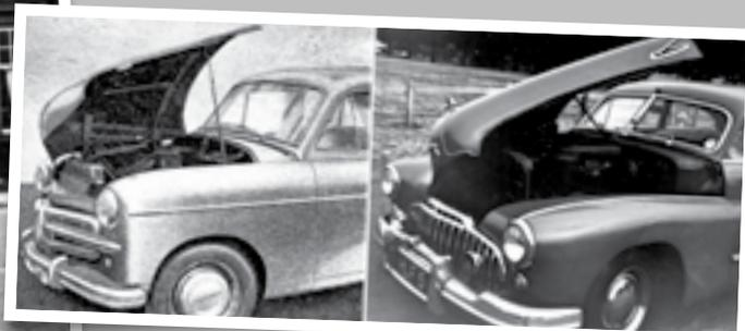
Early E-type Vauxhall bonnets opened from either side, a GM novelty shared with this 1946 Buick (right) by means of a combined hinge and fastener.
