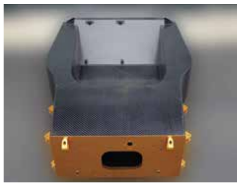
▲ ToPCaT carbon chassis lightweight structure
